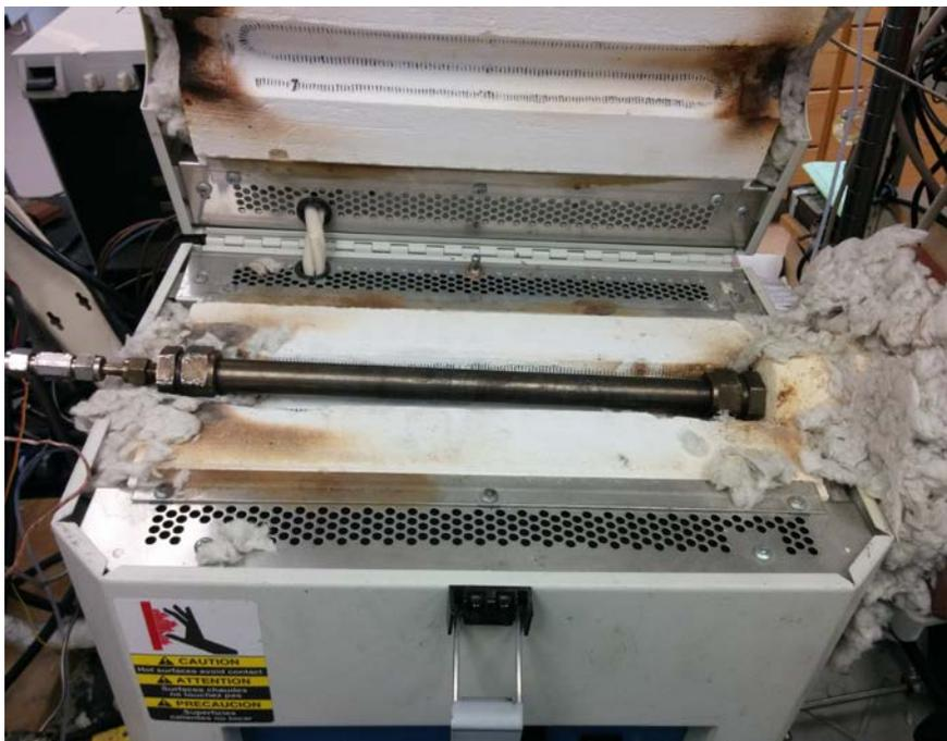
**Figure 18:** Reactor tube inside the furnace
