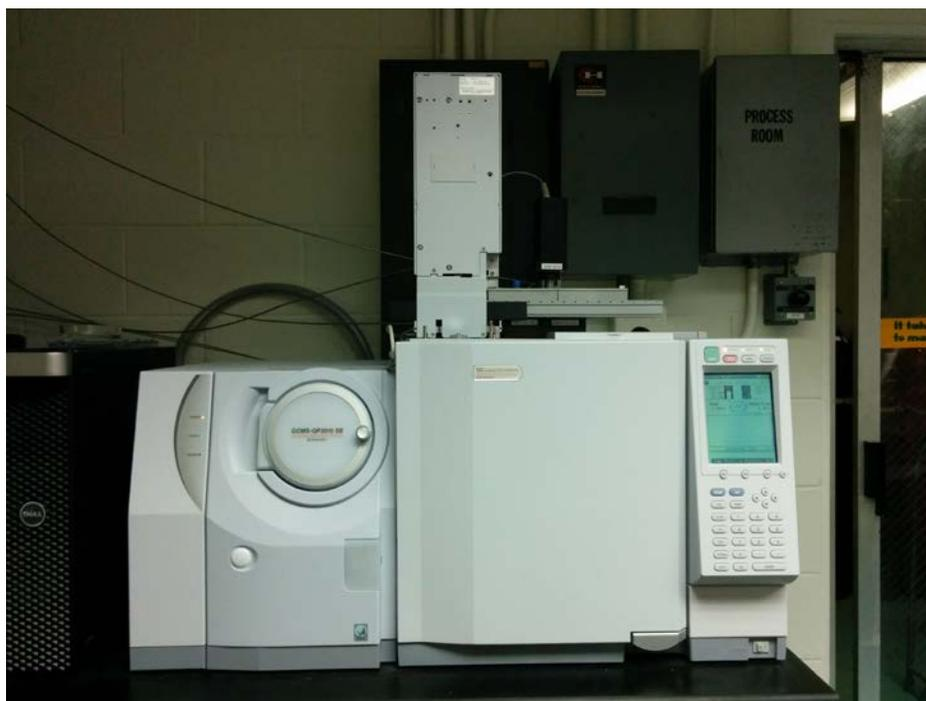
**Figure 24:** WPI's Godard Hall gas chromatography and mass spectrometry
