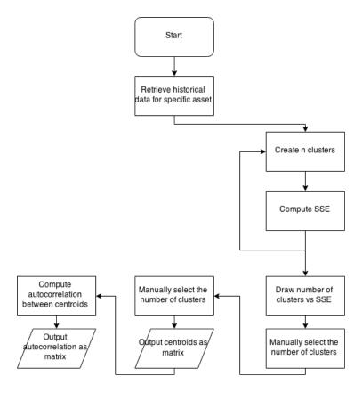
Figure 78: K Means Clustering Flowchart
