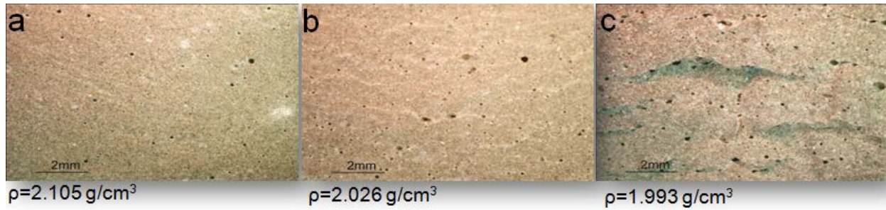
Figure 25: Comparison of microstructure and density among (a) pure cement, (b) 10% ARW Type I dross and (c) 20% ARW Type II dross.
