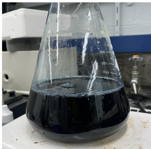
Figure 7: Coomassie Blue G-250 solution being mixed on a continuous stirring apparatus.
