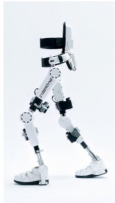
Figure 6: HAL for Lower Limbs (24)
