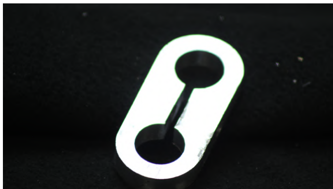
Figure 4.11: Pipe Clamps are used to clamp the inner rigid rods with the hollow tubes
