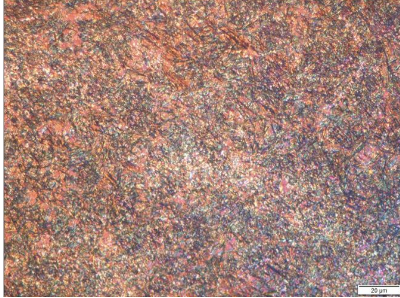
Figure 6: Optical microscope image showing a tint etched sample at 500x magnification. The sample was austempered at 240 °C for 10 minutes.
