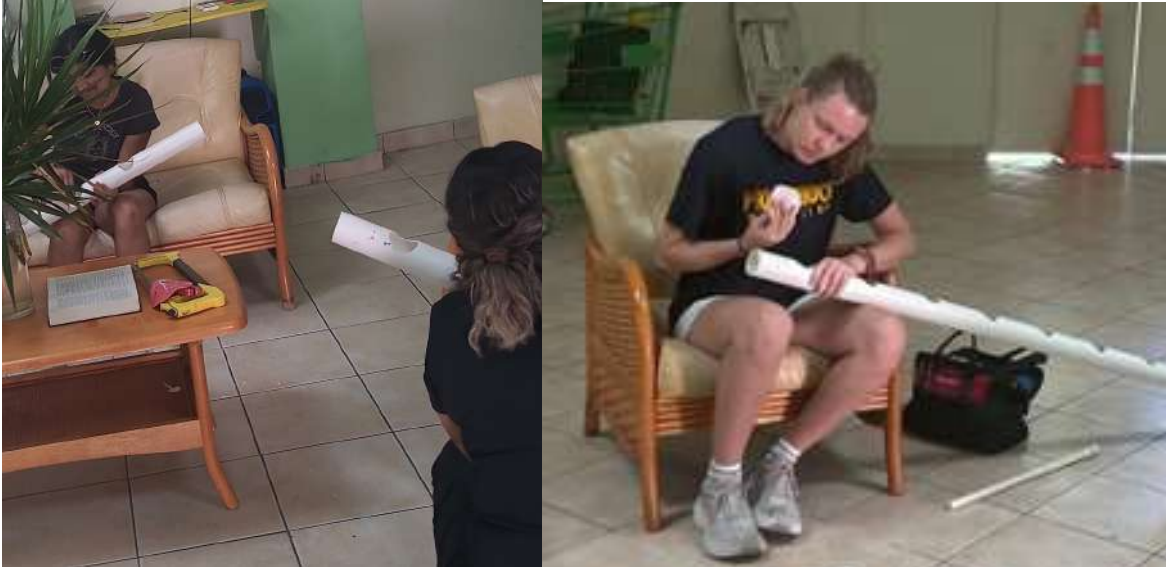
Figure 30: Glory Rodriguez, Rayna Jacob, and Brooke Struble sanding the holes in PVC pipes meant to hold plants in the hydroponic garden.
