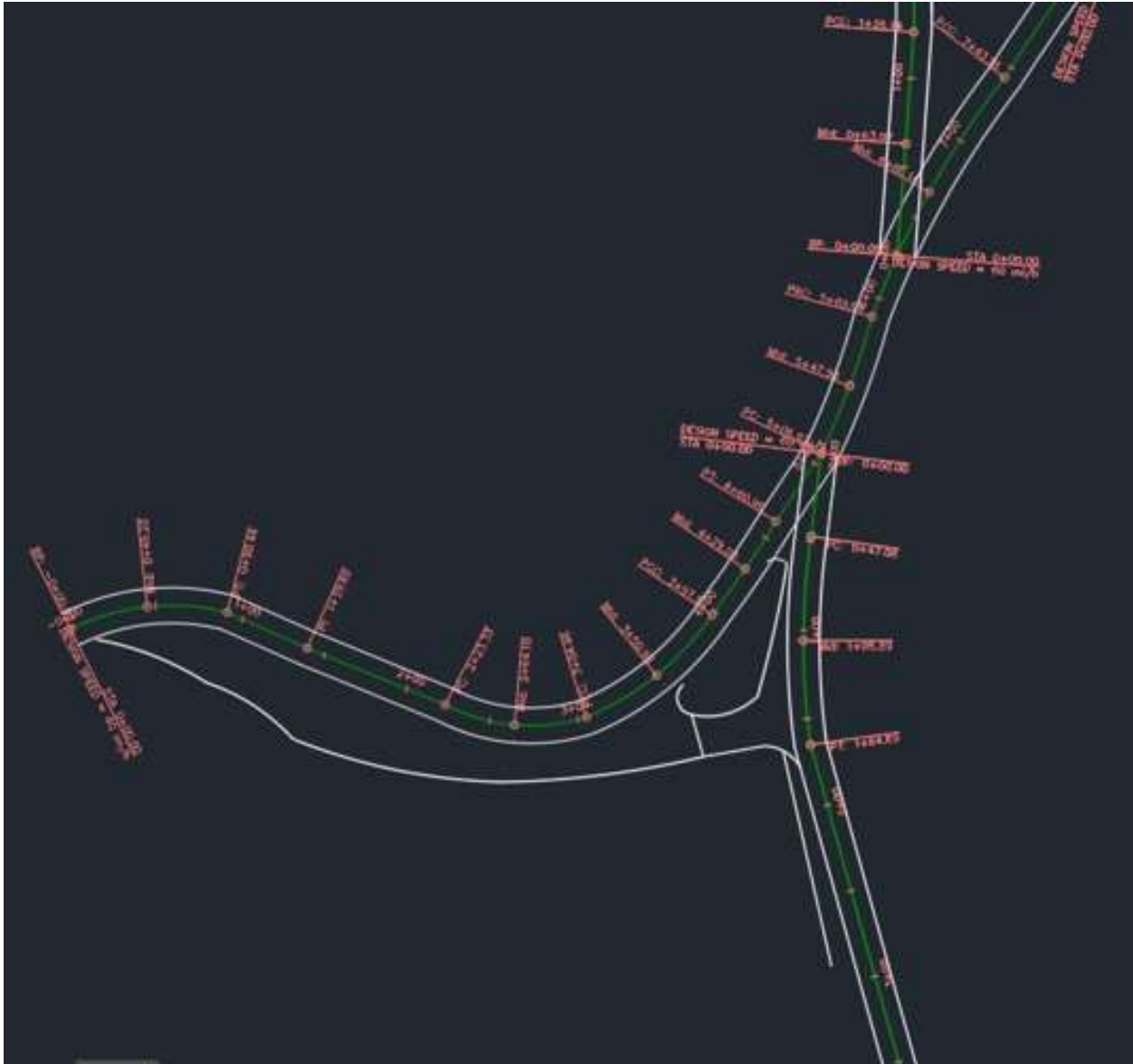
Figures 14a and 14b. The Civil3D renderings of the Centerbridge Group, LLC plans for the roadways in the EHVD with aerial image overlay (14a) and without (14b).
