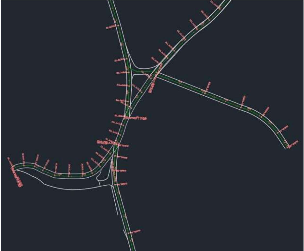
Figures 17a and 17b. Civil3D renderings of the minimal impact roadway design for the EHVD with aerial imagery (17a) and without (17b). This design eases the curve off of the East Haddam Swing Bridge and creates a designated drop-off lane for pedestrians.
