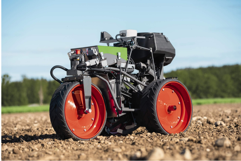
Figure 15: Trike System with One Steerable Wheel
