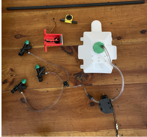
Figure 22: Spray-Bar System from “Car-Snow Clearing Drone” (5L water tank, pump, flat fan nozzles, actuated spray bar mechanism)
