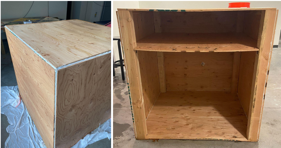
Figure 35 & 36: Weather-Proofed Hub and Hub Interior, respectively
