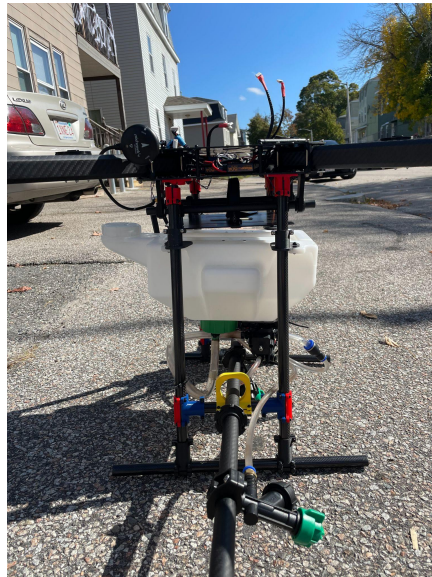
Figure 2: Snow-Clearing MQP Spraying System
