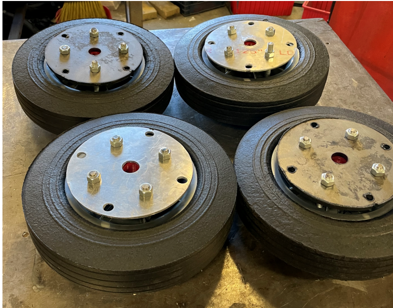
Figure 21: Completed Wheel Hub Assembly
