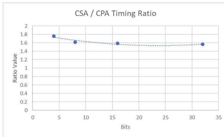
Figure 3.10. Ratio of Carry Select Adder over CPA Timing.
