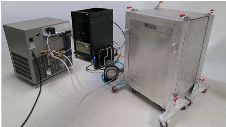
Figure 1: DD110M Neutron Generator manufactured by Adelphi Technologies for use in WPI's radiation laboratory.
