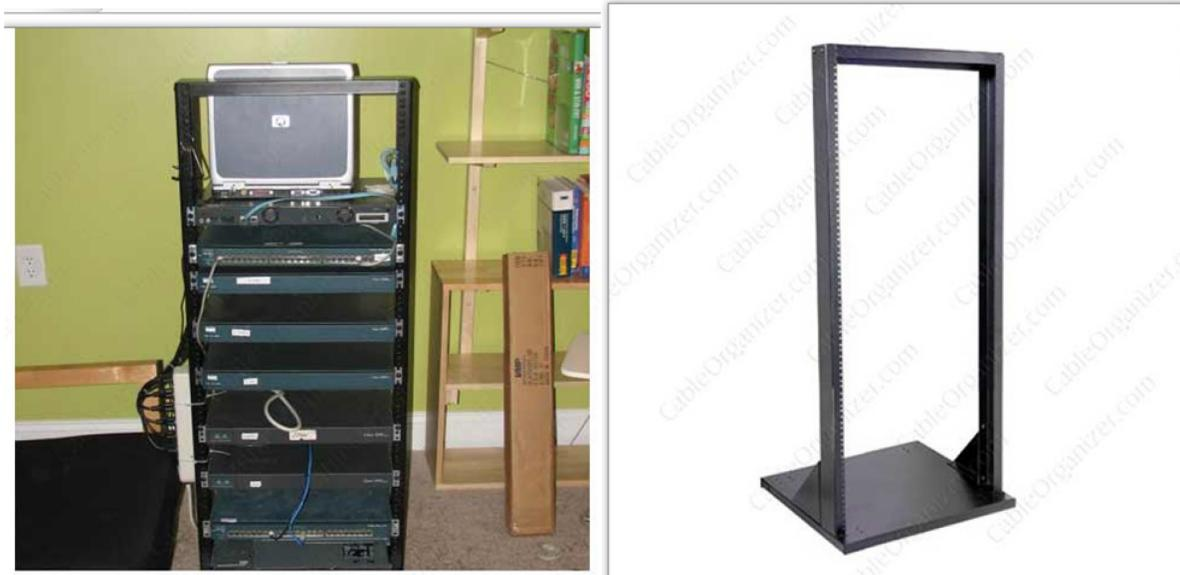
**Figure 3.1 Two-Post Economy Open Frame Rack (Left) and Frame (Right).**
