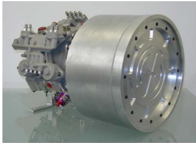
c. Full KERS system with vacuum chamber
