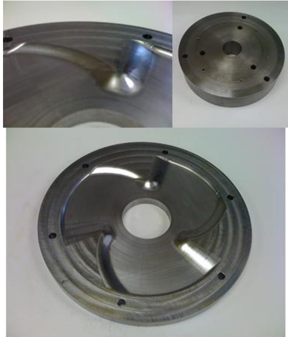
Figure 3.8: Finished cam and flywheel
