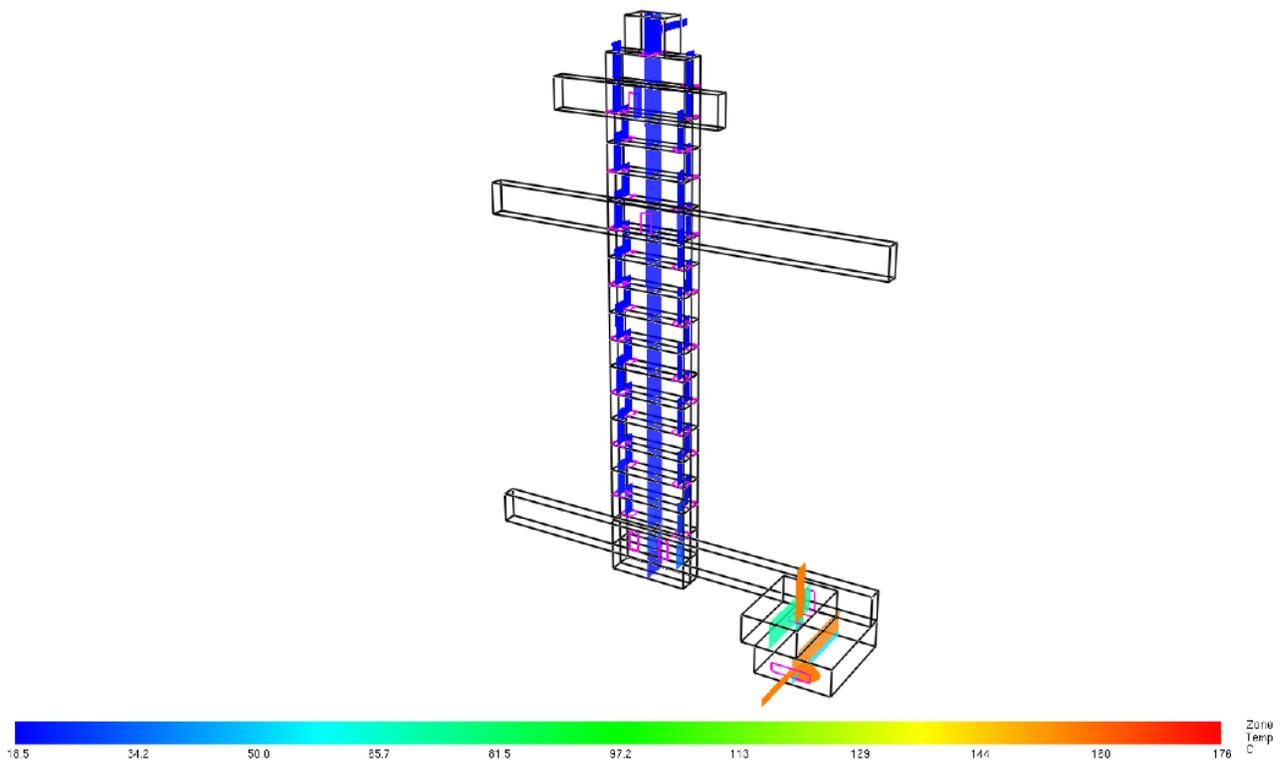
*Figure 30: Temperature of Upper/Lower Layer at 240 seconds*
