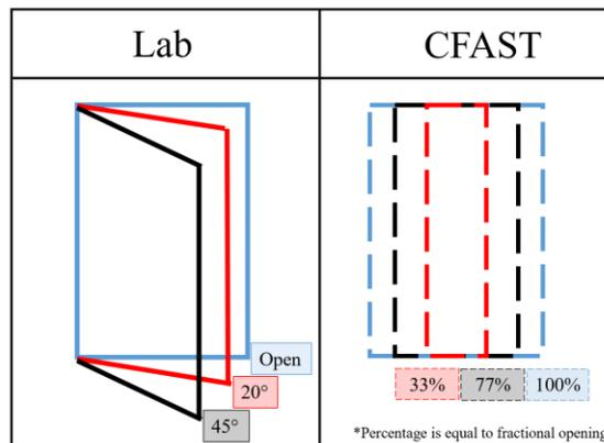
Figure 18: Door Configuration between our lab tests and CFAST tests
