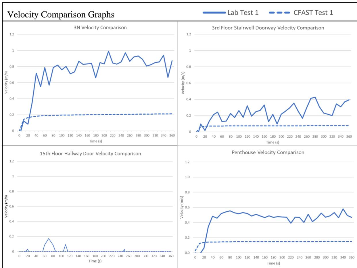
Figure 25: Velocity Comparison for Open Doors Test
