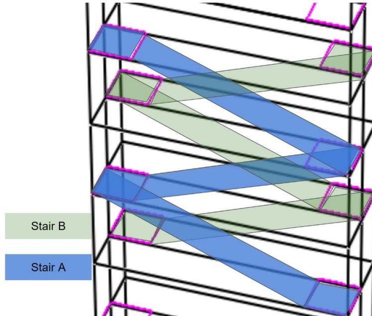
Figure 17: CFAST Vent Layout for Stairwell Configuration
