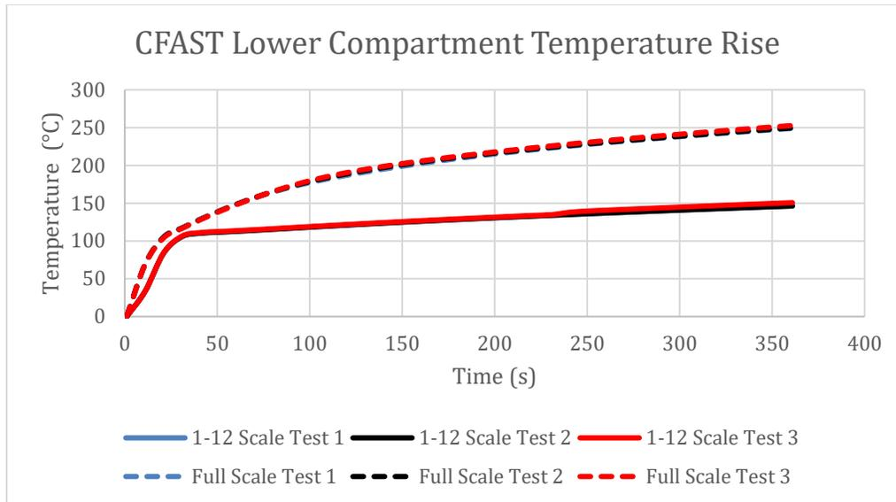
Figure 24: Lower Compartment Temperature Rise for the Full-Scale Model
