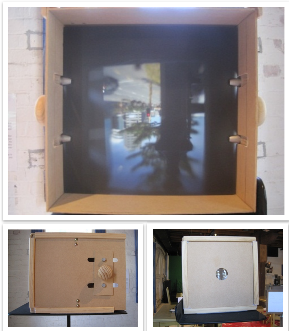
Figure 14: Camera obscura model. Top: Translucent viewing screen of inverted image. Bottom Left: Side view of focus adjustment handles. Bottom Right: View of aperture and lens on front of model.
