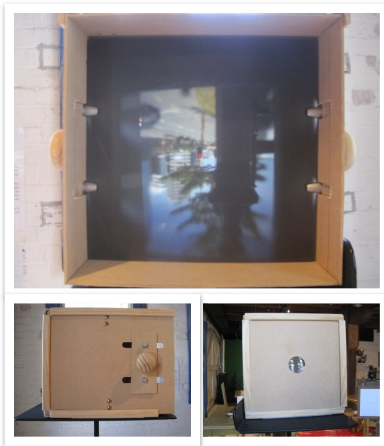
Figure II: Camera obscura model. Top: Translucent viewing screen showing an inverted image. Bottom Left: Side view of focus adjustment handles. Bottom Right: View of aperture and lens on front of model.
