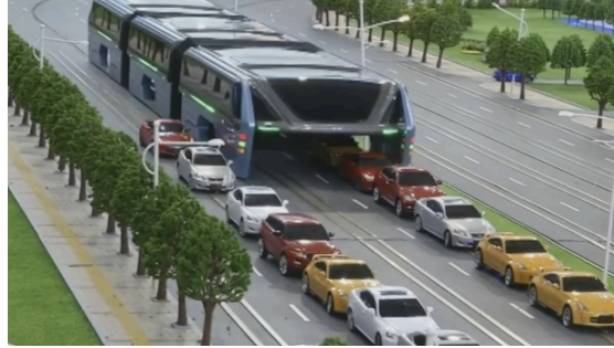
Figure 1: A model prototype of the "straddling bus" concept (Ylanan, 2016)
