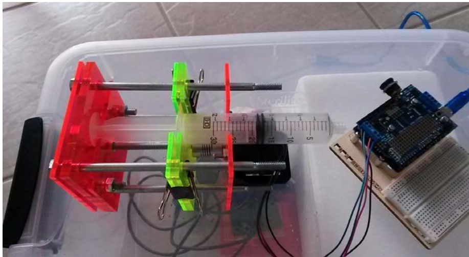
Figure 23: Model 2 of the Laser Cut Syringe Pump
