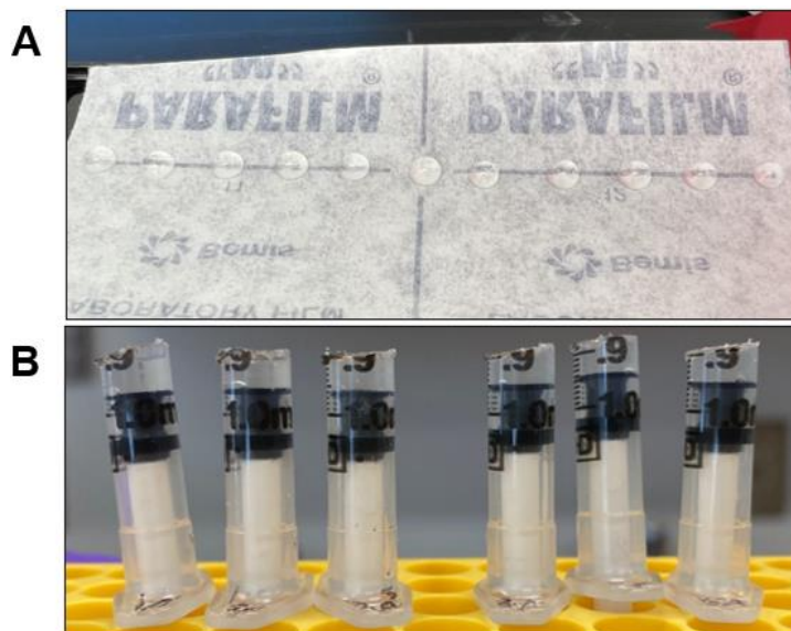
Figure 16: (A) The droplet on parafilm gelation set-up for the 20 \mu L hydrogels, and (B) the cutoff syringe gelation set-up for the 50 \mu L hydrogels.
