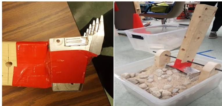
*Figure 11 Bucket Excavator Prototype*
