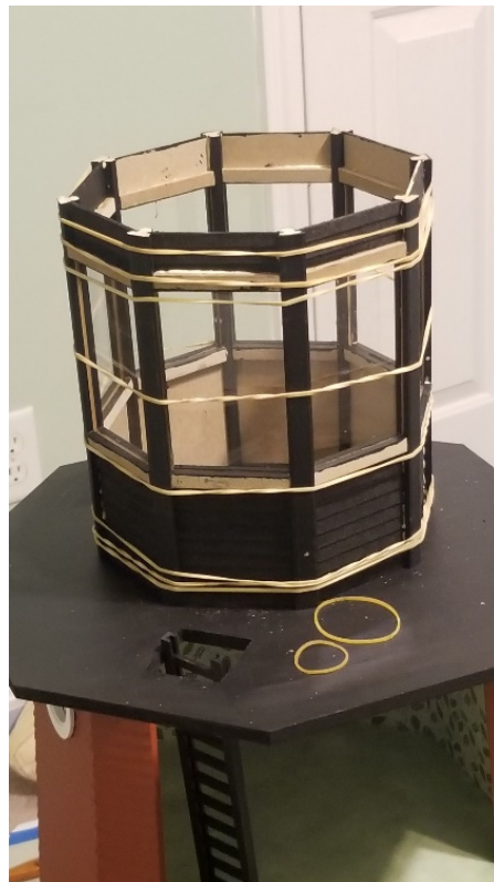
Figure 4-8 Rubber bands clamp the light housing while it dries.
