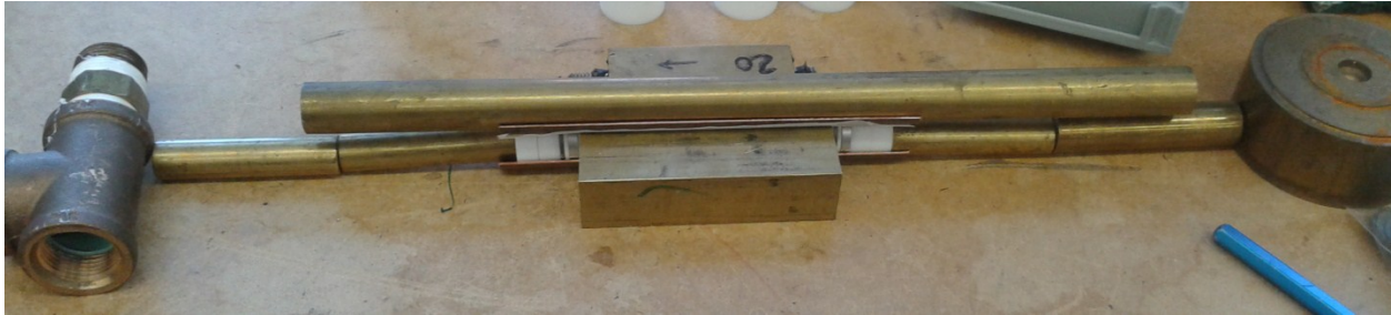
Figure 30: Weighing Down a Pump Section to Ensure Contact with the Busline
