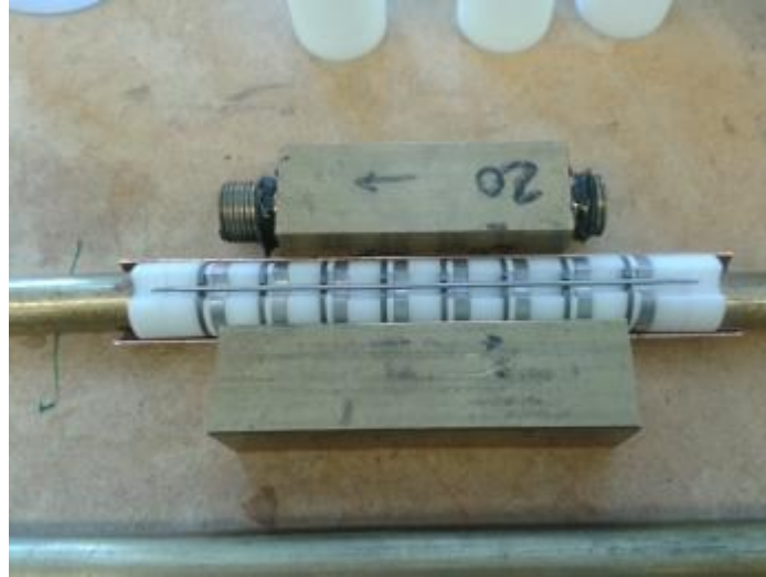
Figure 29: Pump Section Assembly Using a Cradle
