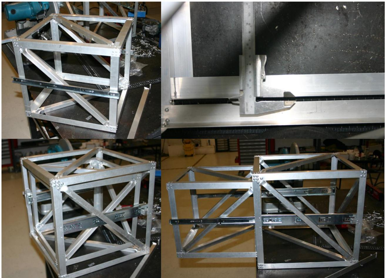
Figure 59: Rail attachment process, clearances and final design
