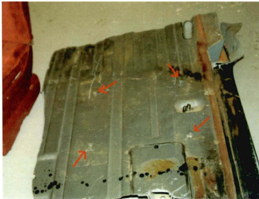
Figure 5.4: Four-Floor Pan Hole Marked By Red Arrows
