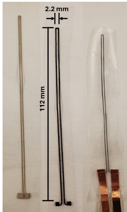
Figure (2.2) (From left to right) Silver, Carbon, and ELMNT sensors before attachment.
