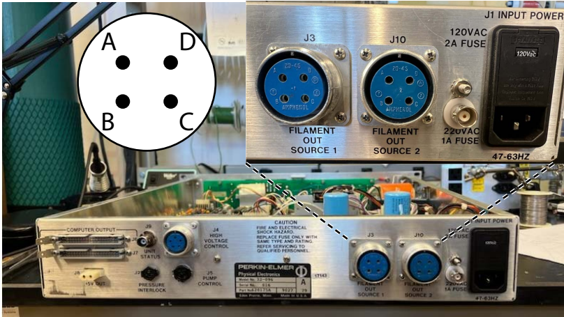
Figure D.1. Exterior view of the back of the 32-096 X-ray control box where the filament cable pin connections for both J10 and J3 are A-D clockwise respectively.
