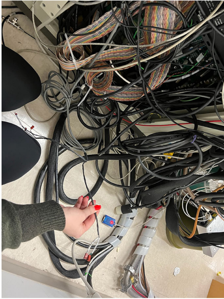
Figure D.6. A252-J13 and A252-J14 cables unplugged. The other ones in the bundle remain unplugged (except J36 2-pin male connector discussed in §9.4.4), while J13 and J14 plug into board A252.
