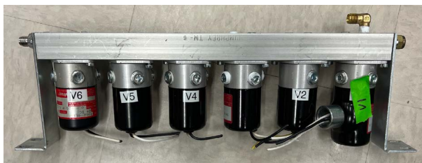
Figure D.4. Photo of the original XPS valve manifold for which we clipped the cable connections and took offline.
