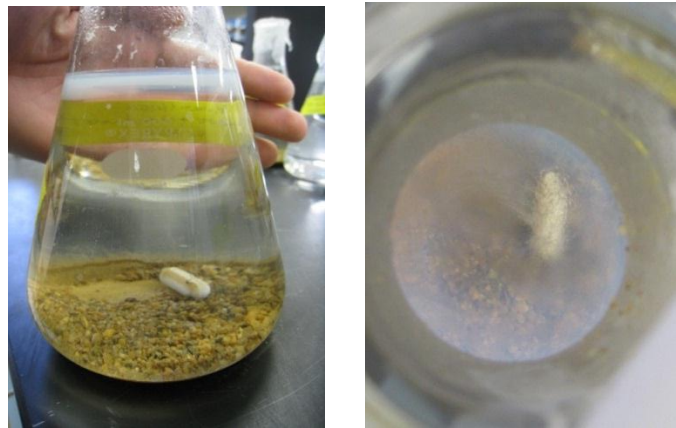
Figure: 31 Sand first with 500mL seawater and 2.0mL of COREXIT followed by the addition of 0.0394 inch sand
