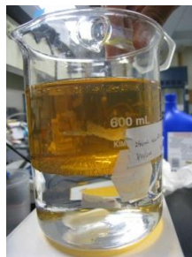
Figure: 62 Diagram of 500mL Seawater mixed with 250mL oil and 2.0mL COREXIT 9500.A
