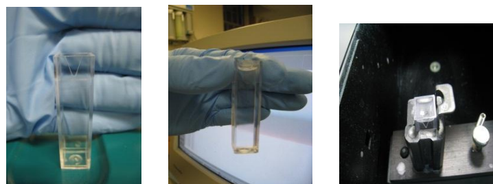
Figure 4.9 The Cuvette used for the light spectroscopy of the bottom reading of 500mL Seawater and COREXIT 9500A (1.0mL)
