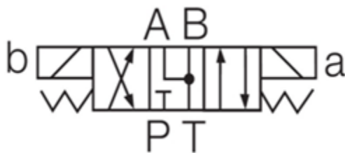
Figure 19: Unmodified control valve schematic
