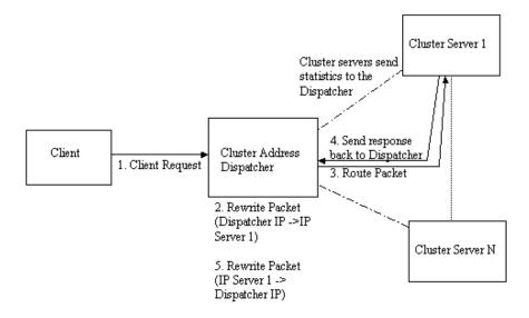
Figure 2.4: Dispatcher Based Redirection: Packet Double Rewriting
