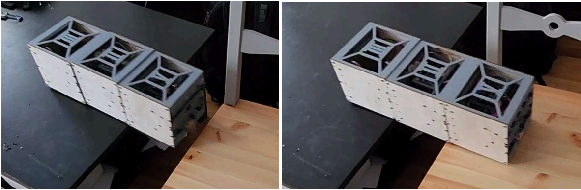
Figure 37: Three Cubes Bridging a One Robot Wide Gap
