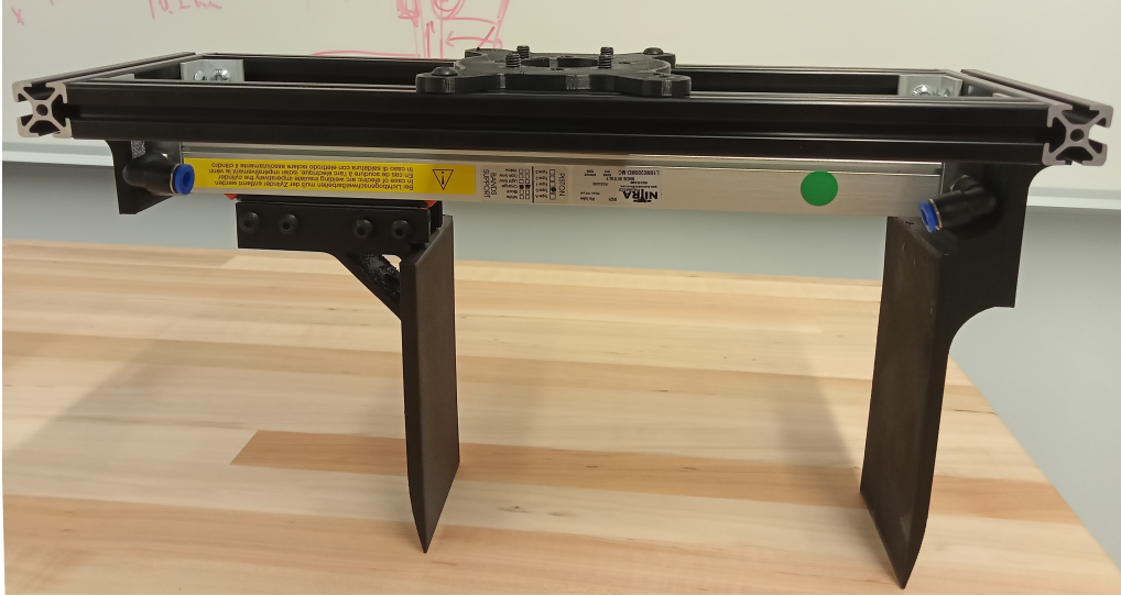
Figure 3.3: Mechanical assembly of the envelope gripper
