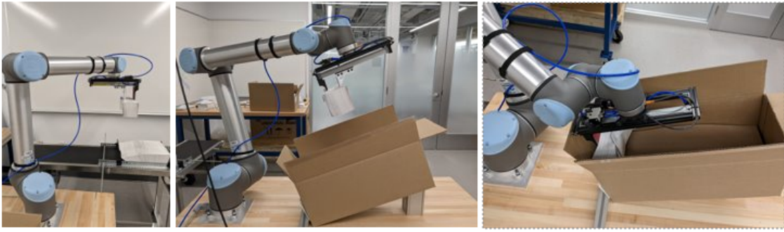
Figure 5.5: Step-by-step depiction of the envelope pick and place
