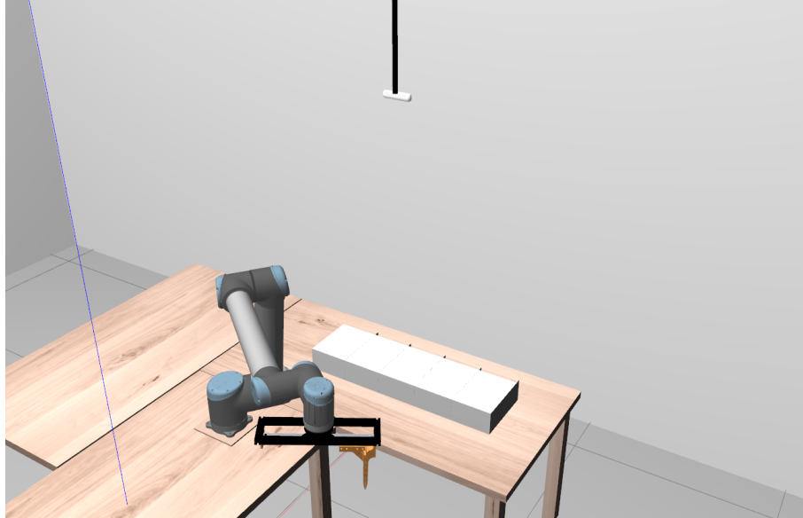
Figure 4.1: Simulation of a virtual RGB-D camera mounted from the ceiling which captures images of envelope stacks
