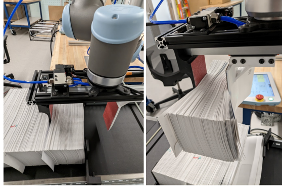
Figure 6.10: Failure to slide the notch into the stack due to inadequate force applied during sliding motion
