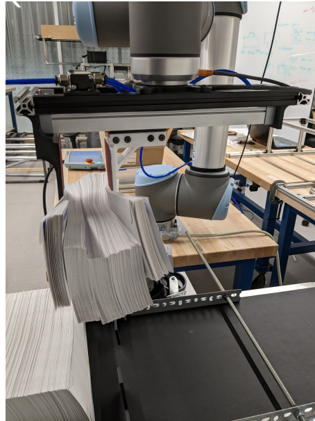
Figure 6.7: Picking failure caused by a combination of the other failures or inadequate pressure
