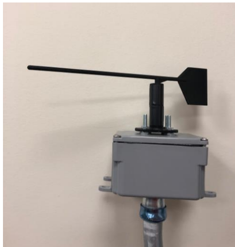
Figure 5: Wind Vane Structure and Enclosure
