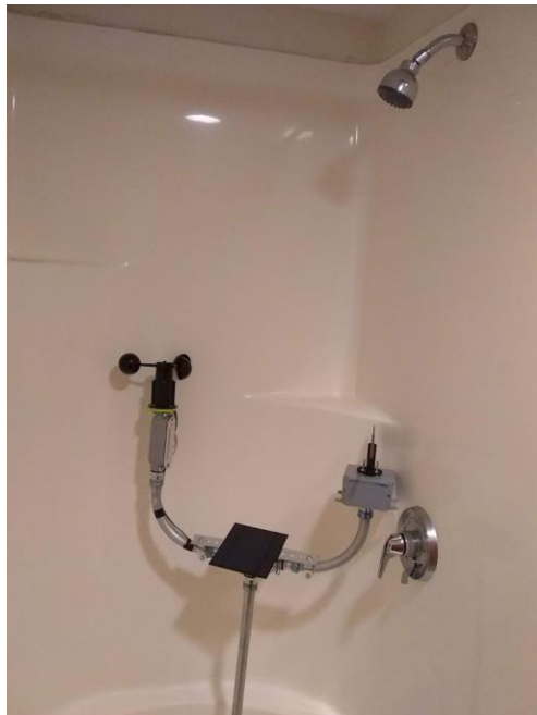
Figure 33: The Waterproofness Testing Environment
