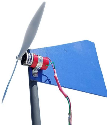
Figure 11: First Do-It-Yourself Mini Wind Turbine Example
