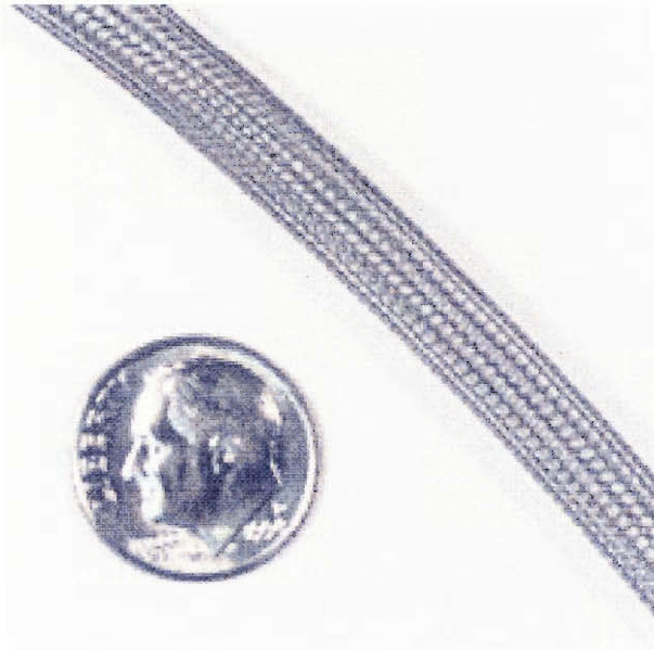
Fig. 1.2: Fine NiTi shape memory or superelastic wires can be woven into cylindrical shapes for various applications. One such application is vascular stents to reinforce blood vessels. The stent is squeezed and inserted through a cannula into the proper location in the blood vessel. Upon warming above its transformation temperature, the stent returns to its trained cylindrical shape and provides reinforcement to the walls of the blood vessel. ( http://www.sma-inc.com/WovenWire.html )
