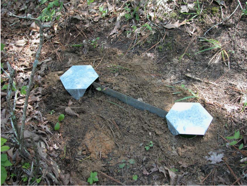
Pitfall traps separated by steel guide vane Source: MacGown, Joe. "Insect Collection Methods"
