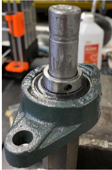
Figures 34 and 35: Damaged shaft and Machined shaft with key
