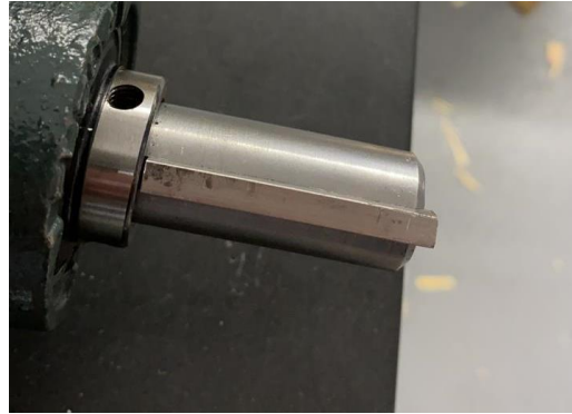
Figures 34 and 35: Damaged shaft and Machined shaft with key
