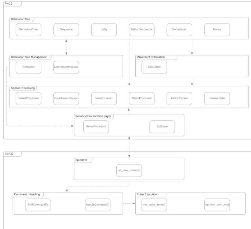
**Figure 5.10 Software UML Module Diagram**
