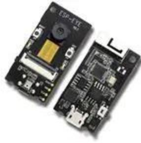
**Figure 4.11 ESP-EYE Camera Board**
