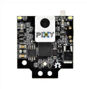
**Figure 4.12 Pixy2CMUcam5 Image Sensor**
