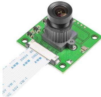
**Figure 4.13 Arducam with M12 lens module**
