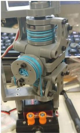
Figure 5.2 Servo driven test fixture
