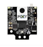
Figure 4.12 Pixy2CMUcam5 Image Sensor
