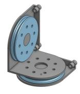
(a) CAD model of a pulley pair
