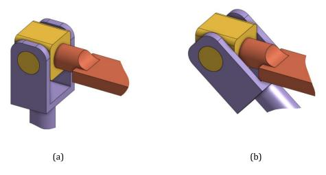
Figure 4.9 Zoomed View of U-Joint Platform Joint. Shown: yoke (purple), spider (yellow), platform pin (red)
