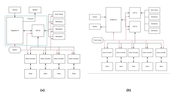
Figure 4.18 Initial and Final Electrical System Diagrams
