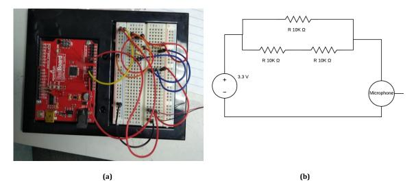
Figure 5.6 Microphone Test Circuit with Arduino. Physical circuit(a) and Circuit Diagram (b)
