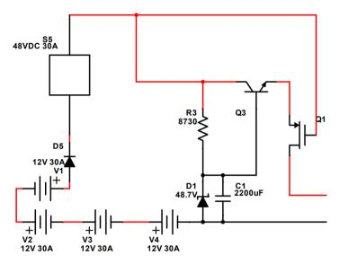
Figure 4.19 Power Supply and Delivery Circuit Diagram
