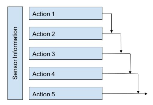
Figure 4.31 Diagram of a Subsumption System
