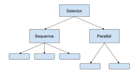
Figure 4.33 Diagram of a Behavior Tree
