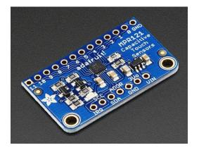
Figure 4.17 Adafruit 12-key Capacitive Touch Sensor
