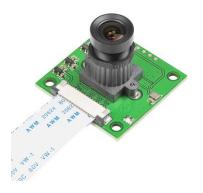
Figure 4.13 Arducam with M12 lens module
