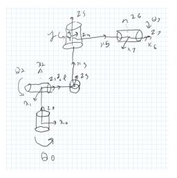
Figure 4.1 Kinematic outline of the neck and head mechanism
