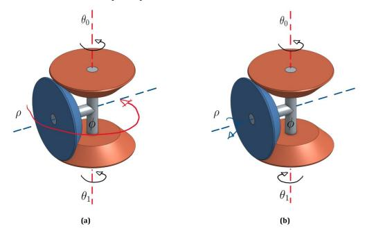
Figure 4.2 Simultaneous (a) and differential (b) input rotation of the differential mechanism
