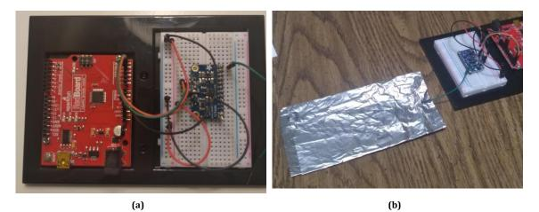
Figure 5.8 Touch Sensor Circuit and Test Setup
