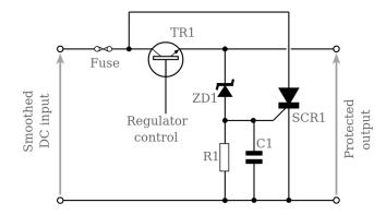
Figure 4.22 SCR Crowbar Circuit
