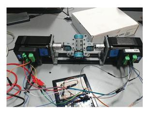
Figure 5.3 Stepper driven test fixture
