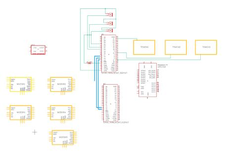
Figure 5.5 Electrical System Schematic Ported to Autodesk Eagle
