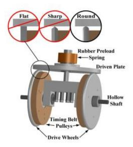
Figure 4.3 Diagram of Friction Wheel Differential
