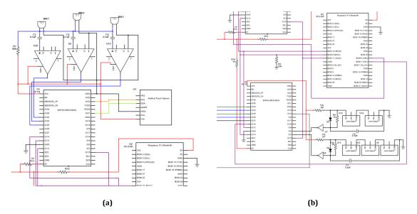
Figure 4.24 Processor Circuit. Sensor ESP32 (a). Motor Control ESP32 and Raspberry Pi (b)
