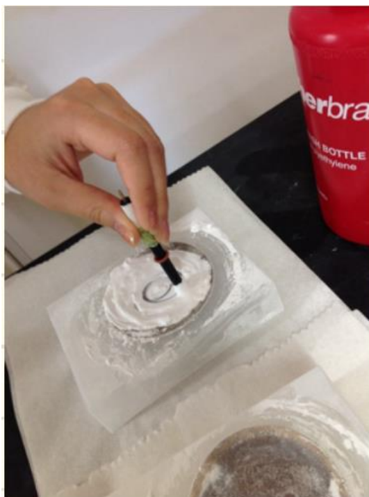
2. Glassy carbon electrode coated with multi-walled carbon nanotubes Figure 7. GCE is being polished using alumina polish.
