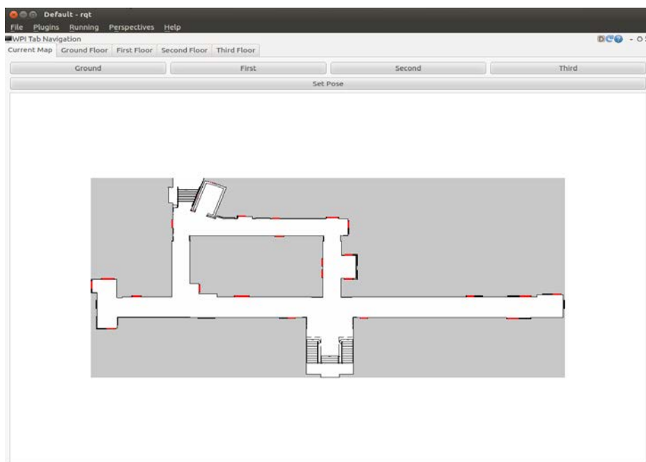
Figure 62: Navigation rqt plugin (ground floor)
