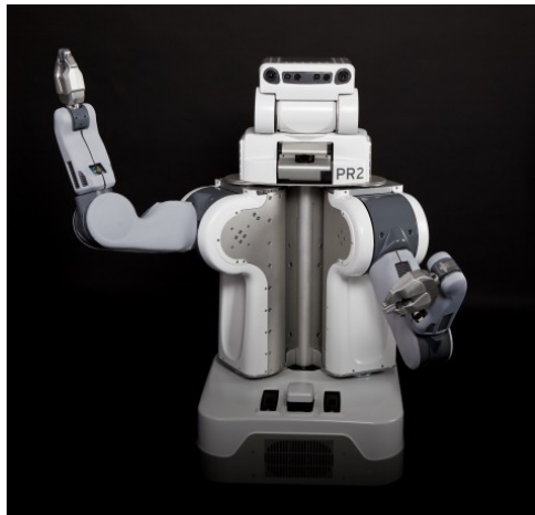
Figure 7: Front view of PR2 with multitude of sensors (Garage, 2014)
