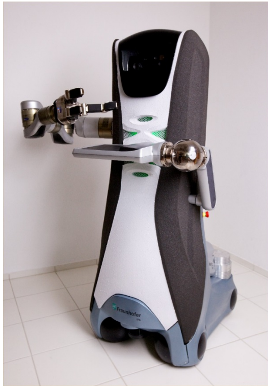
Figure 6: Care-O-bot 3, displaying its adjustable tray and robotic arm (Automation, 2013)
