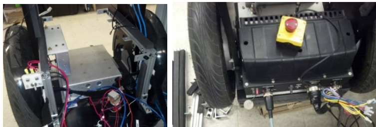
Figure 1: Original control box (Left) and new control box (right)
