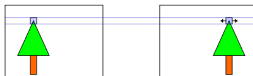
Figure 17: Images from each camera after rectification (Gerig, 2012)
