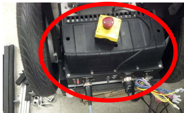
Figure 29: Segway Control box after servicing
