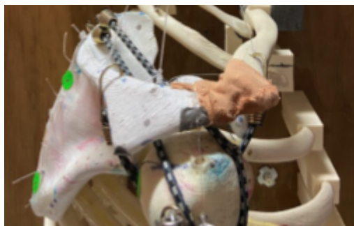
Figure 22: KT Tape used to replicate the acromioclavicular ligament capsule.
