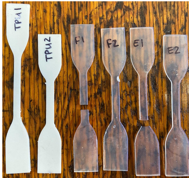
Figure 29: Comparisons of the TPU, flexible, and elastic materials. TPU1, F1, and E1 were subjected to tensile testing, while TPU2, F2, and E2 were not.
