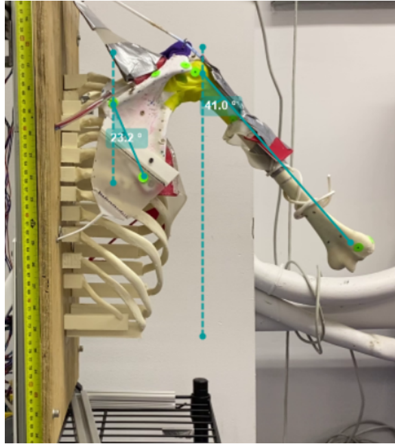
Figure 36: The videos of the abduction movement were analyzed using the “measure angle from vertical” tool in Kinovea.
