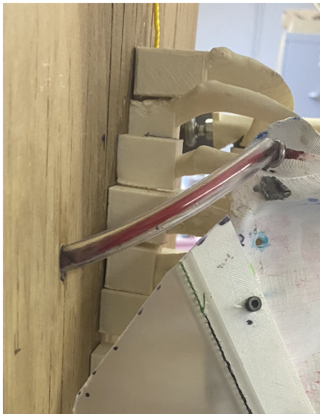
Figure 32: Bowden cable at use in the model on the supraspinatus muscle.
