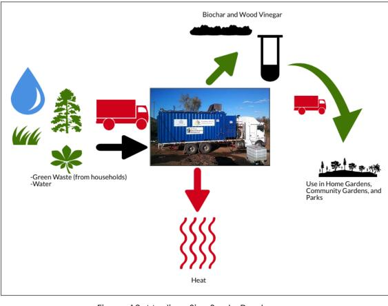
Figure 18: Medium Size Scale Pyrolyzer
