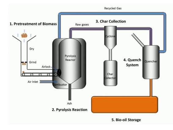
Figure 10: Biomaterial Production Process (Biofuel Journal, 2018)
