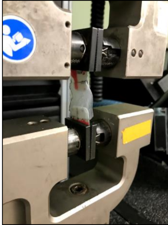
Figure 4.2: Uniaxial Instron test of hydrated rice paper with Velcro grips
