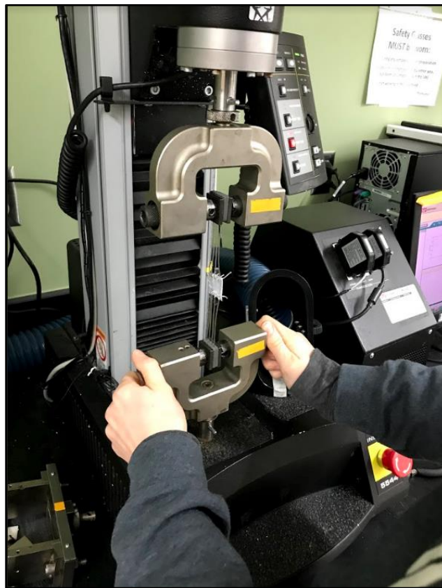
Figure 4.5: Uniaxial test of hydrated rice paper using initial rake prototype design
