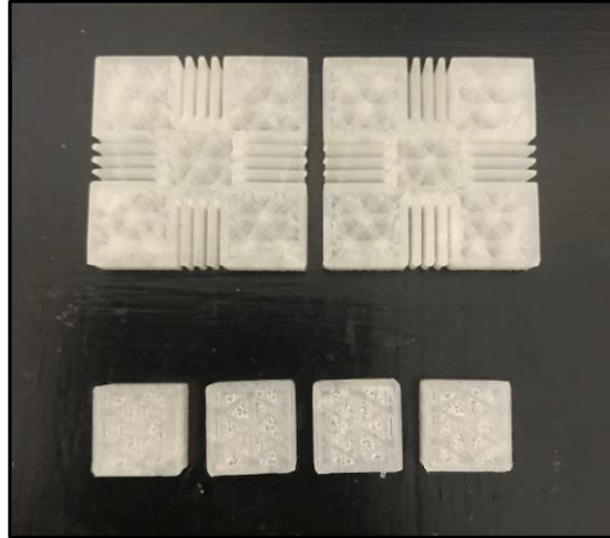
Figure 4.15: First prototype of tine spacers and loading platform
