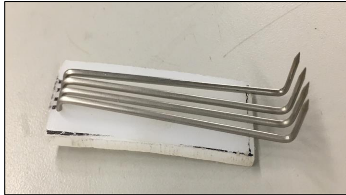
Figure 4.12: First prototype of the final grip design produced on a large scale. The tines are 1.5mm diameter stainless steel mounted in a 0.95 cm thickness base of UHMWPE
