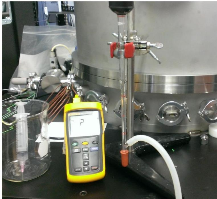
**Figure 22:** Bubble-O-Meter up close.
