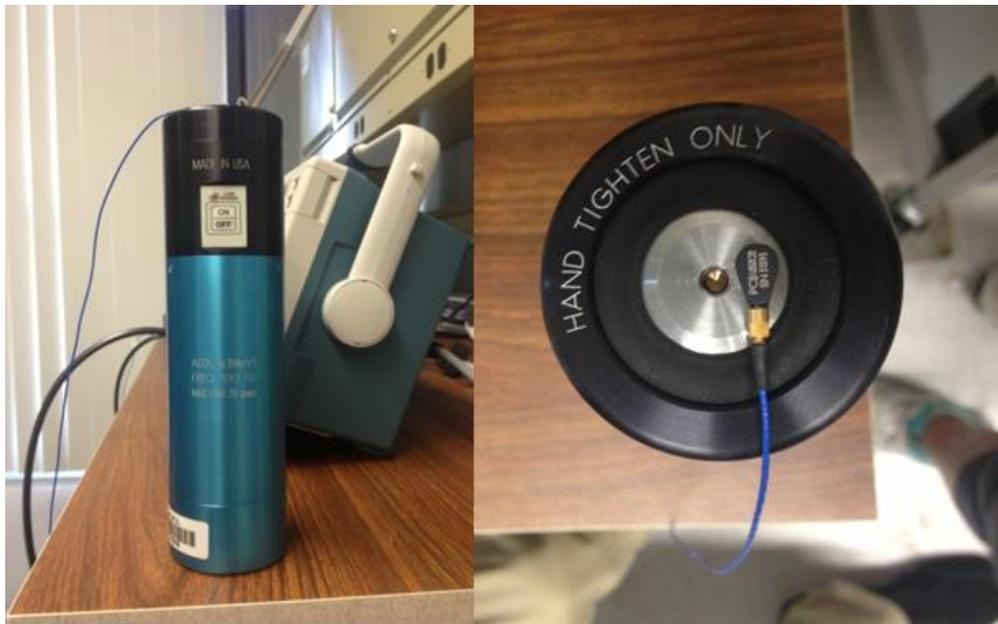
**Figure 9:** Accelerometer calibration using hand-held shaker.
