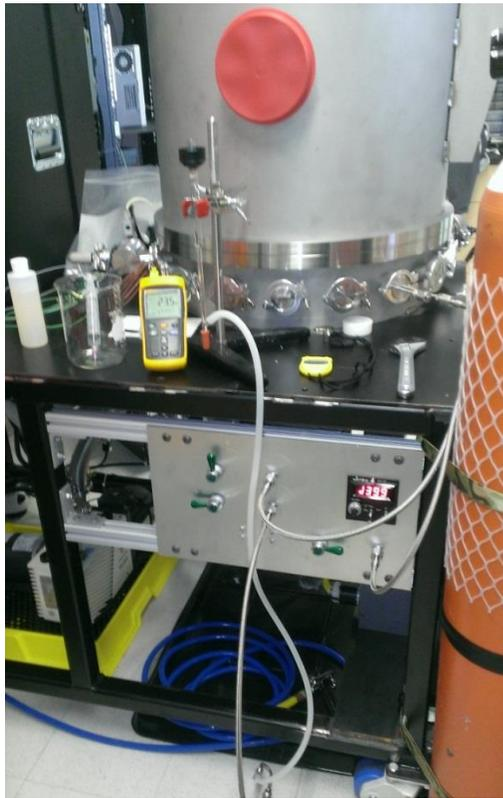
**Figure 21:** Mass flow system calibration setup.
