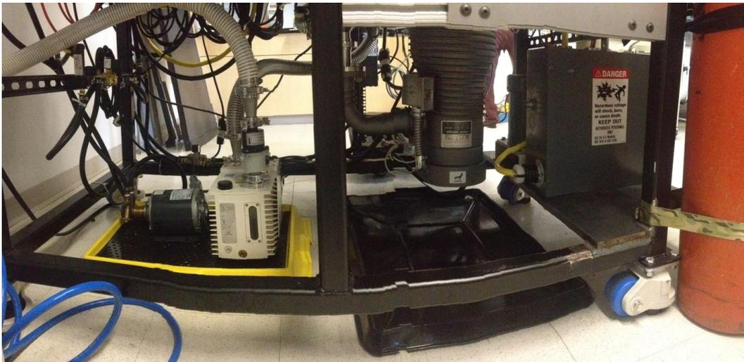
**Figure 7:** Vacuum pump located below table in SVF-2.
