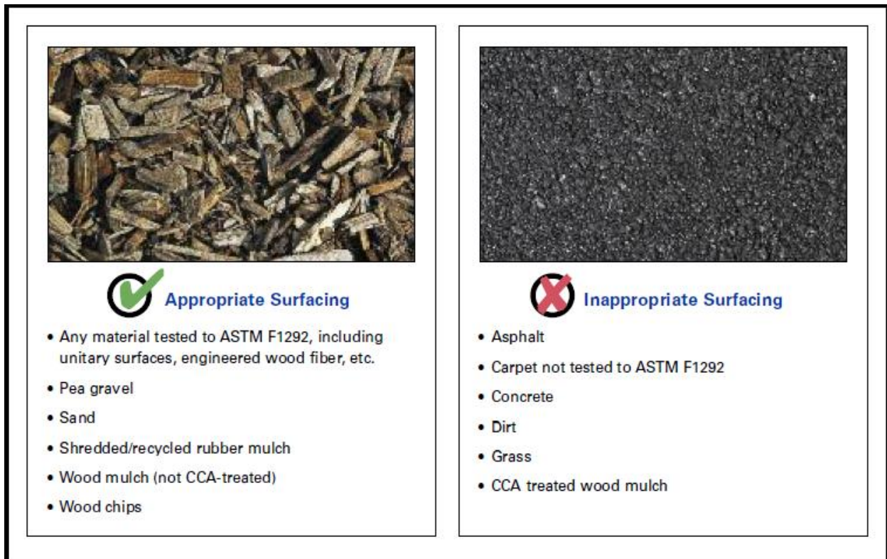
Figure 16: Example Surfacing Materials (CPSC, 2010, Section 2.4.1)
