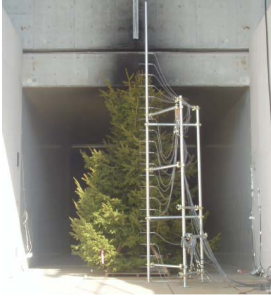
Figure 2.14 – Location of the tree within the wind tunnel. The cross-section measured 4m x 4m.
