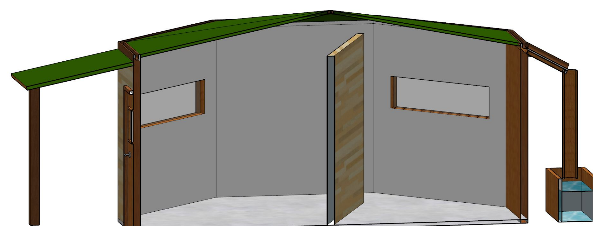
The low pitched roof, with a slope of 6/12, allows wind to pass over the top with ease.
