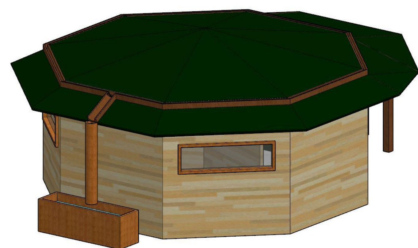
The roof uses a system of gutters to collect and funnel water into a cement storage unit.
