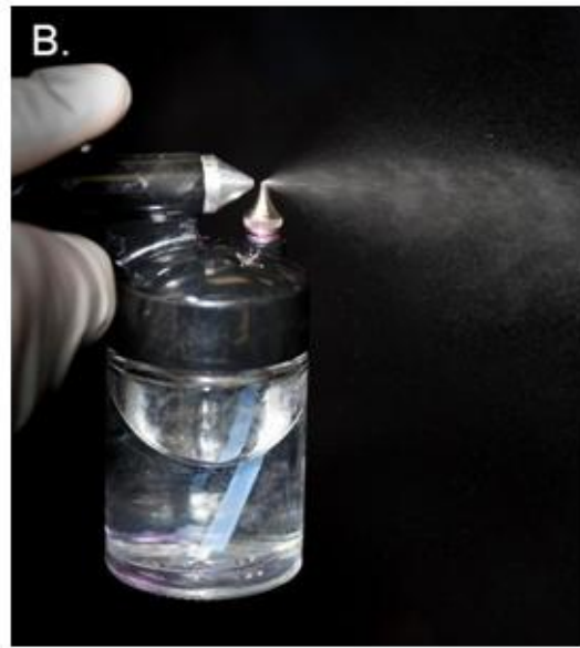
Figure 10. Preval Spray Gun (A) Close-up of Atomization; Badger Model 250 Airbrush (B) Close-up of Atomization
