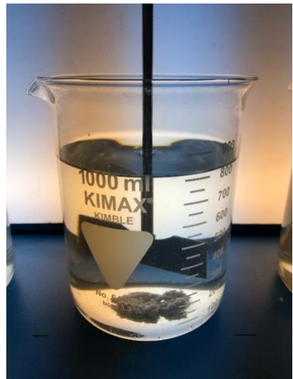
Figure 20: (a) Jar testing experimental set-up; (b) 2 \text{ mg} \cdot \text{L}^{-1} \text{ FeCl}_3 during rapid mix period; (c) 2 \text{ mg} \cdot \text{L}^{-1} \text{ FeCl}_3 during flocculation period; (d) 2 \text{ mg} \cdot \text{L}^{-1} \text{ FeCl}_3 during settling period
