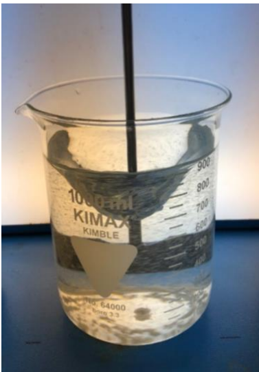
Figure 20: (a) Jar testing experimental set-up; (b) 2 \text{ mg} \cdot \text{L}^{-1} \text{ FeCl}_3 during rapid mix period; (c) 2 \text{ mg} \cdot \text{L}^{-1} \text{ FeCl}_3 during flocculation period; (d) 2 \text{ mg} \cdot \text{L}^{-1} \text{ FeCl}_3 during settling period
