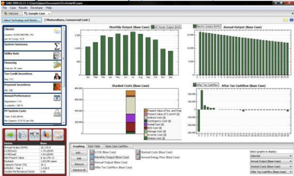
Figure 216. Performance Analysis, First Solar Tilted 42°, Oriented South -8°
