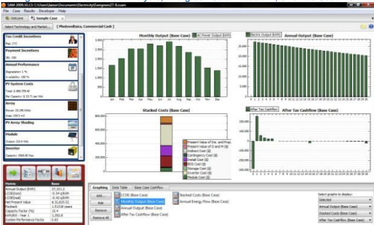
Figure 209. Performance Analysis, Evergreen Solar Tilted 42°, Oriented South
