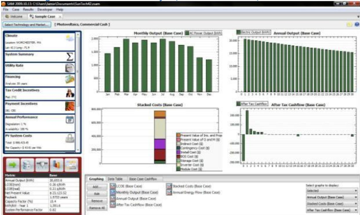
Figure 204. Performance Analysis, SunTech Tilted 42°, Oriented South -8°
