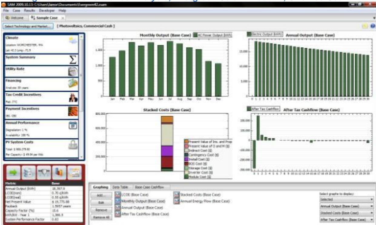
Figure 210. Performance Analysis, Evergreen Solar Tilted 42°, Oriented South -8°
