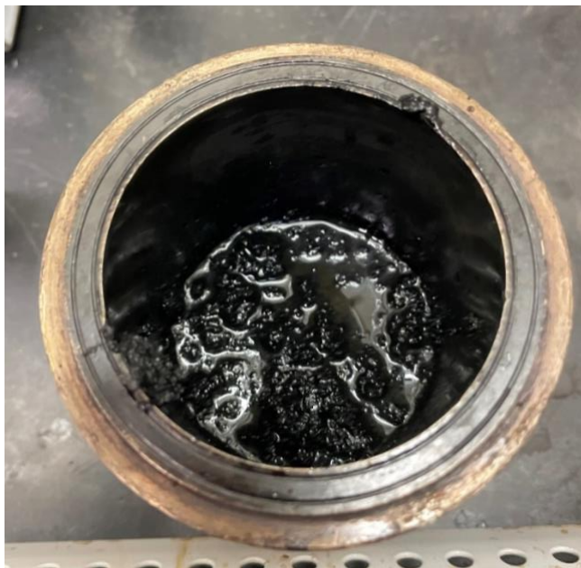
Top-down view of reactor bottom after depressurization and reactor head removal. Clumps of solid phase product are visible floating in the aqueous phase.
