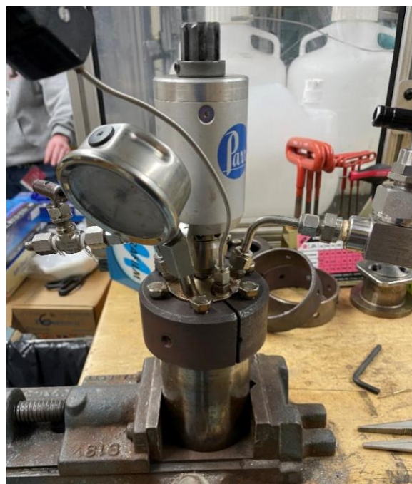
Benchtop removal of reactor collar. The inner collar is visible, securing the head and bottom of the reactor together. The collar is fastened with six bolts.
