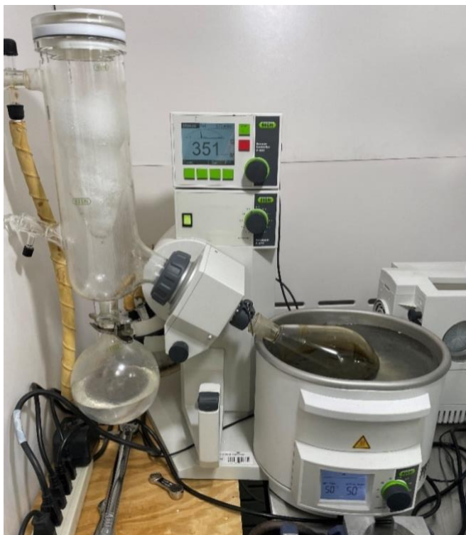
Rotary evaporation of oil/acetone mixture.
