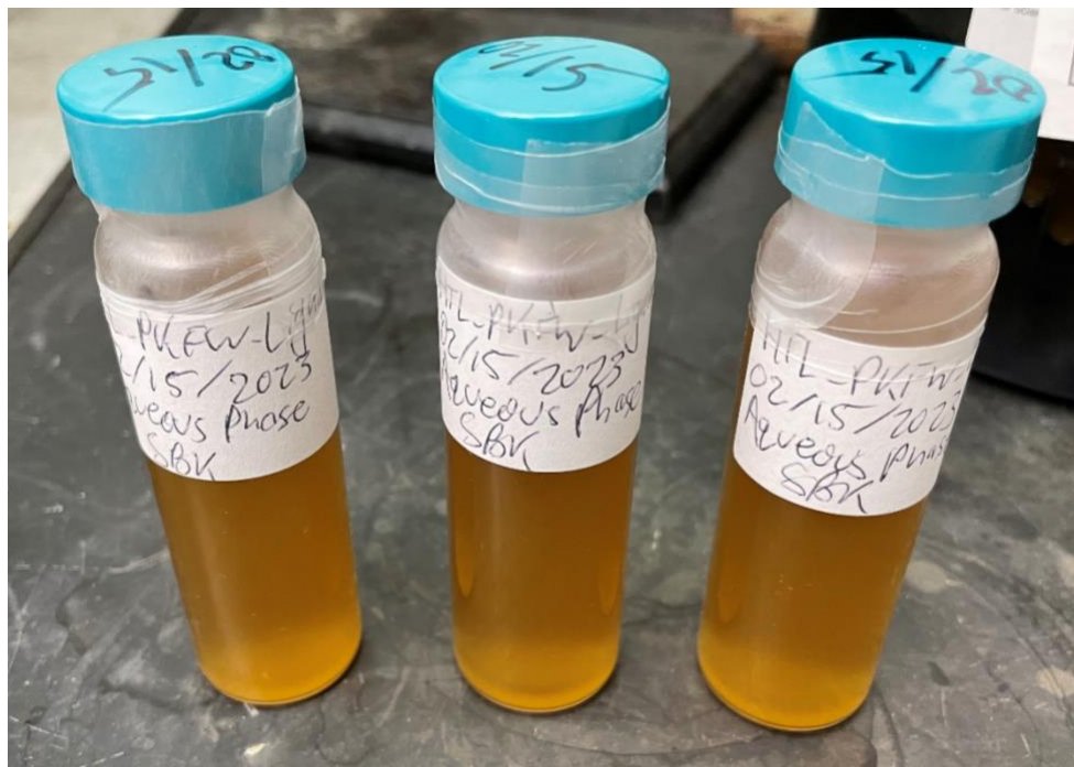
Isolated aqueous phase after vacuum filtration, stored in three individual 5-dram vials. All vials pictured were sourced from the same reaction.
